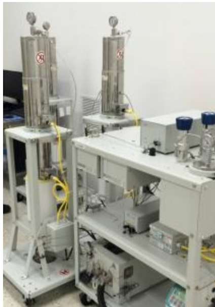
Figure 13. Aphria's Waters CO 2 critical extraction setup
